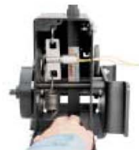
The test arm is pulled down to release the fire vent doors without breaking the ETL ®* .
