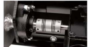
Rotary limit switch is coupled to the outboard shaft on the reducer to limit travel in both directions.
