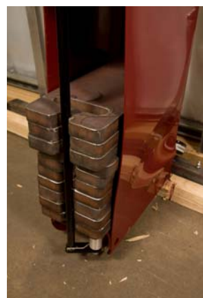
Test #1 – Bottom shelf weight movement and deformation post test.
